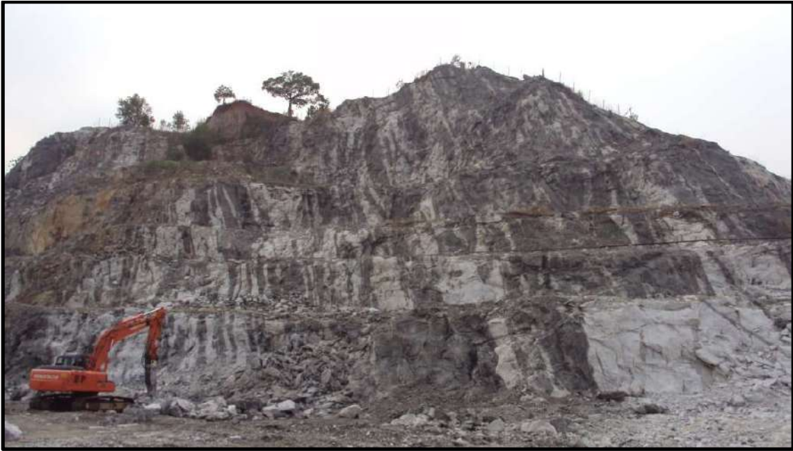
Photograph showing the Bench Type Mining
